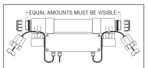
IMPORTANT: Ensure that equal amounts of the quartz sleeve are visible at each end of the unit before fitting the locking nuts.
